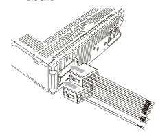
2 Check the car's wiring carefully and connect them to the supplied male connector.
